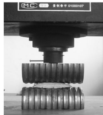
图1 杉木制材板皮辊压图 Figure 1 The rolling pressure figure of sawmill slab of Chinese fir
