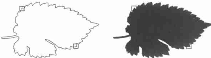
沿叶缘滑动矩形窗口采样 sampling with a rectangular window along the edge
