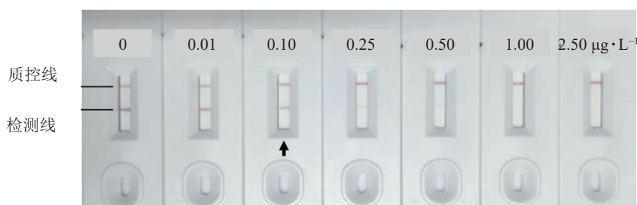
图 5 免疫层析法对黄曲霉毒素 B 1 的定性检测限 Figure 5 Detection limits of immunochromatographic assay for aflatoxin B 1
